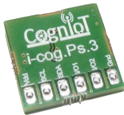
Bottom View. iCog Ps.3 Pressure Sensor
